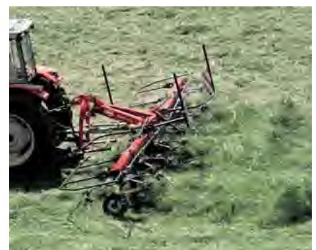
The Fanex 763 with 7.6 m working width.
