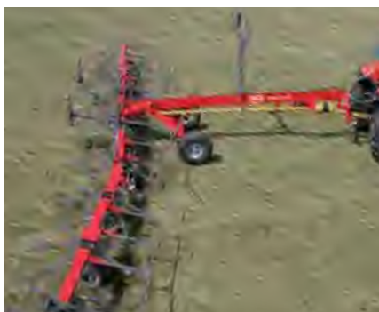
For border tending the 3 outer rotors are pivoted, to secure evenly inward spreading.
