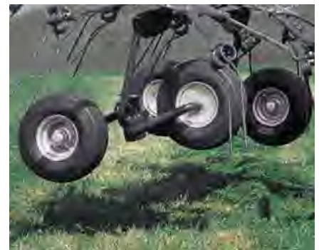
Optional tandem axles enhance ground contour following ability and quiet running.
