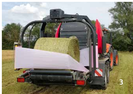
As soon as the bale is transferred away from the baler, the tailgate automatically closes, and baling can resume.
