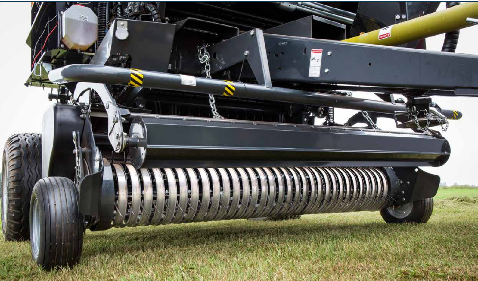
Re-designed large diameter roller crop press facilitates crop flow at high intake speeds.
