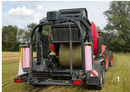
Once the net is applied to the bale the wrapping table moves forward under the tailgate of the baler.
