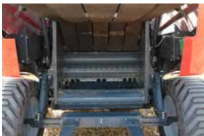
A combination of 5 belts and three rollers provides dense bales with a soft core and an easy bale start.
