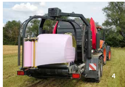
The wrapping table moves rapidly to the pre-stretchers and wrapping starts instantly.
