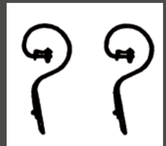
Two rows Straight tines 45 x 10mm
