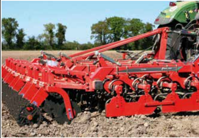
TLG equipped with clod board and combination of crumbler and crosskill roller.
