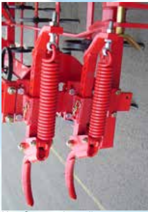
Non-Stop track-eradicators. Possibility to fit 2 units behind each tractor wheels.
