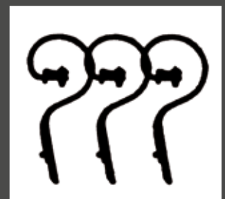
Three rows Straight tines 45 x 10mm
