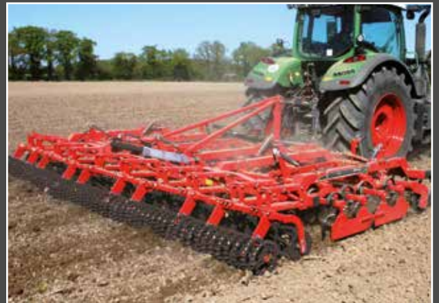
Combination of crumbler and crosskill roller.
