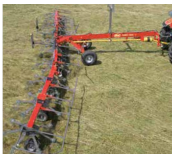
For border tending the 3 outer rotors are pivoted, to secure evenly inward spreading.
