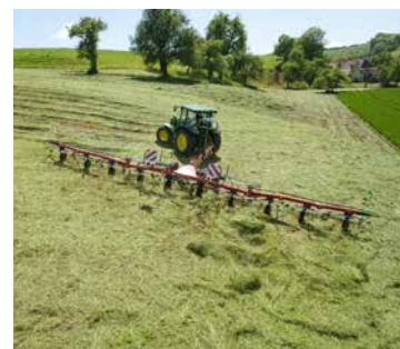
80° turning angle ensures excellent manoeuvrability.
