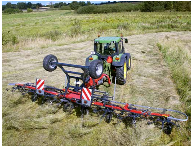
Get the most out of your crop. With border tending you keep the crop inside the field. The tedder is swung hydraulically into border position, conveniently tending the crop away from the border line.
