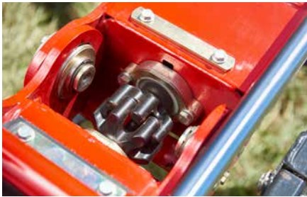
Fanex HexaLink finger clutch permits a 180° folding of the rotors for transport.
