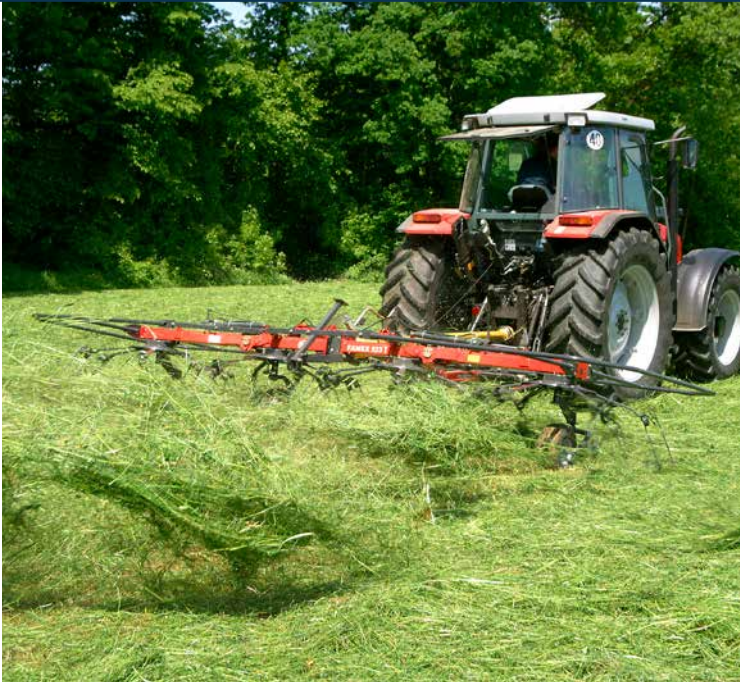
Optional reduction gearbox makes night swath tedding possible.
