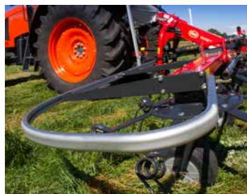
New aluminium rail guards, which are low in weight, but still extremely impact resistant.
