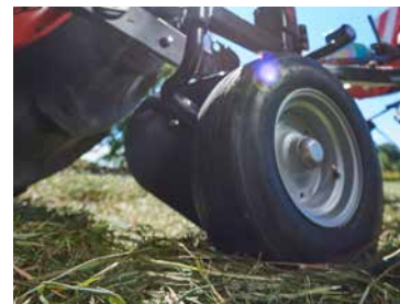
Optional third wheel lead to even more accurate track following and better tedding action.
