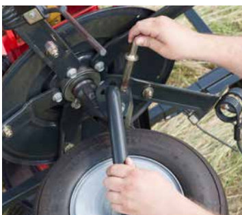
Easy adjustment of spreading angle.
