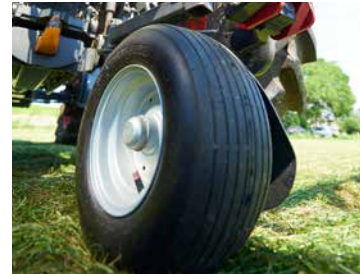
As an option the tedders can be equipped with a third wheel to improve contour followings.
