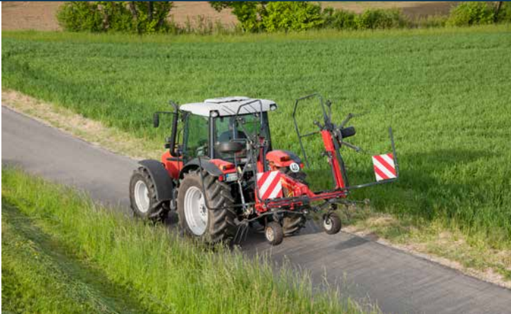
All tedders fold hydraulically from working to transport position and vice versa.
