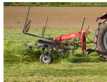
Standard oscillation dampers ensure an even spreading pattern.
