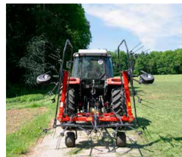
During the hydraulic folding action for transport, the tines are automatically raised.
