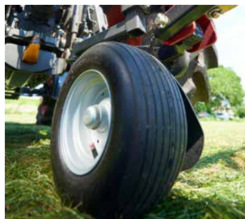
As an option the tedders can be equipped with a third wheel to improve contour followings.
