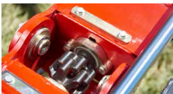
Vicon HexaLink finger clutch permits a 180° folding of the rotors for transport. (Fanex 764, 904 and 1124 (C)).
