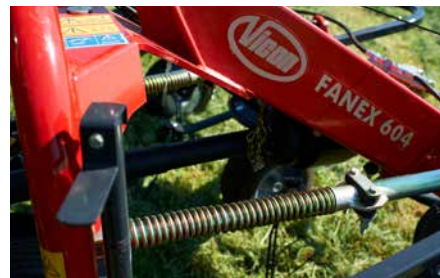
Standard oscillation dampers ensure an even spreading pattern.
