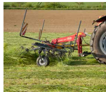
Standard oscillation dampers ensure an even spreading pattern.
