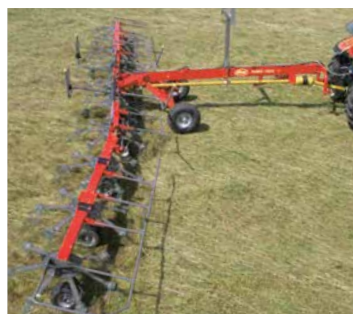
For border tedding the 3 outer rotors are pivoted, to secure evenly inward spreading.
